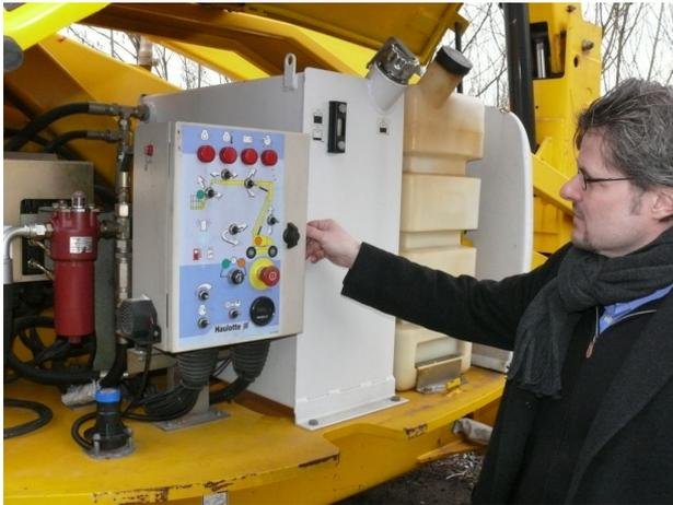
Everyone knows where they stand, because the billing for the working platforms is based on data stored by the Rösler miniDaT system. “By using miniDaTs we have ensured absolute transparency in billing,” says Clemens Streit, Head of Marketing/Sales of the working platform hire company AFI. The Rösler miniDaT system is ultimately a small robust box installed in the platform. Up to five machinery functions can be read using it over 365 working days. The miniDaT can be installed in all mobile and
